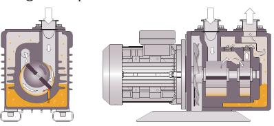
The machine works on the two-stage rotary vane principle.
