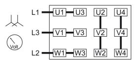
Delta connection, multi-voltage motor (Middle voltage):
