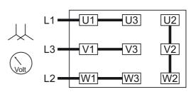
Delta connection, multi-voltage motor (High voltage):
