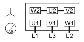
Star-star connection, multi-voltage motor (Low voltage):
