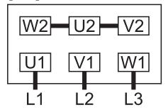
Double star connection, multi-voltage motor (low voltage):
