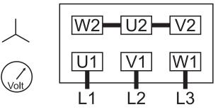
Double star connection, multi-voltage motor (low voltage):
