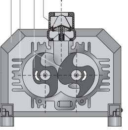
The safety valve (k) on the compressor protects the compressor against overload only. It is **no** pressure limiting device in terms of EN 1012-1 for the pressure system. It is not designed for frequent use and must therefore not be used as a system pressure regulating valve.
