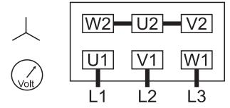
Double star connection, multi-voltage motor (low voltage):
