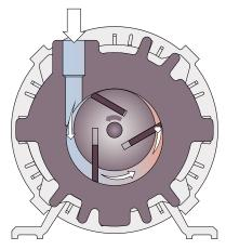
The machine works on the rotary vane principle.
